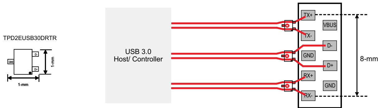
Three TPD2EUSB30 to Protect USB3.0 Class A connector (One Layer Routing)
