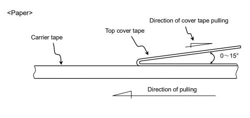
Paper tape should not adhere to top cover tape when pull the cover tape.
