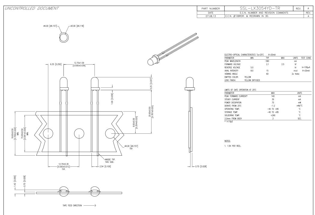
\*UNLESS OTHERWISE SPECIFIED TOLERANCES PER DECIMAL PRECISION ARE: X=±1 (±0.039), X.X=±0.5 (±0.020), X.XX=±0.25 (±0.010), X.XXX=±0.127 (±0.005). LEAD SIZE=±0.05 (±0.002), LEAD LENGTH=±0.75 (±0.030). MIN=  $\frac{+0ECIMAL}{-0.00}$  MAX.=  $\frac{+0.00}{-0.00}$
