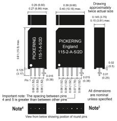
Note4: Pin 3 is round with an outer diameter of 0.0175 (0.44).
