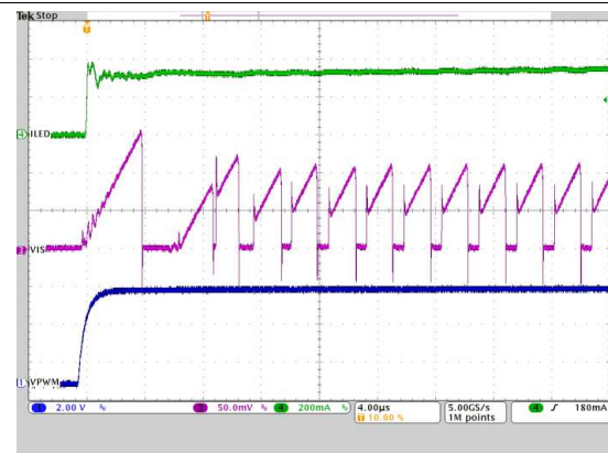
Ch1: External PWM input voltage; Ch3: Switch sense current resistor voltage; Ch4: LED current; Time: 4 μs/div Figure 49. PWM Dimming Transient (Zoomed)
