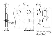
Embossed Carrier Tape Dimensions in mm (not to scale)
