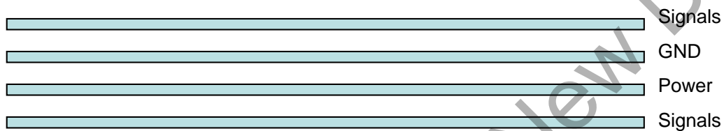
Figure 15: Typical 4-layer PCB construction
