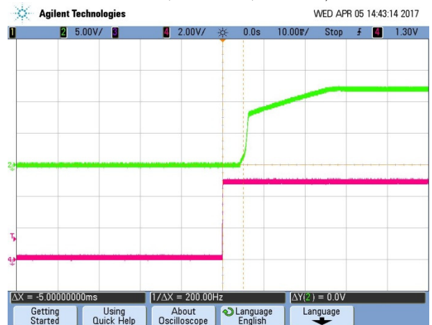
On/Off Enable Delay (Vin = 12V Vout= nom Iload =0A Cload=4700μF CH2: Vout; CH4: Enable; Ta=+25°C)
