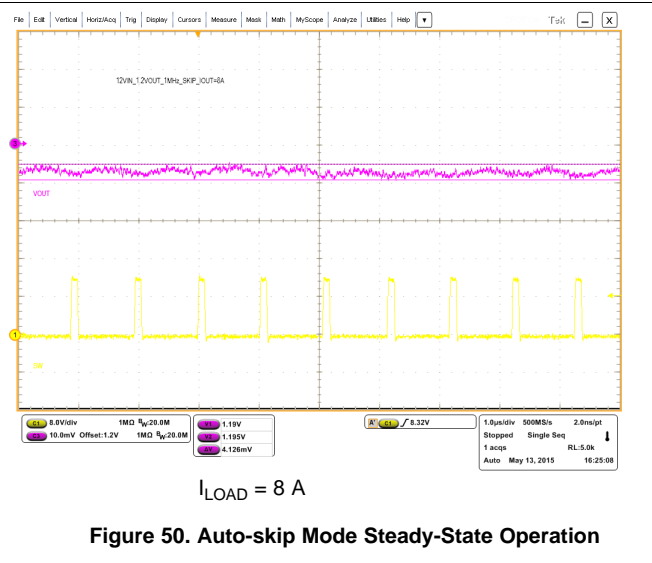
Figure 48. Auto-skip Mode Steady-State Operation
