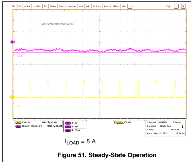
Figure 49. FCCM Steady-State Operation
