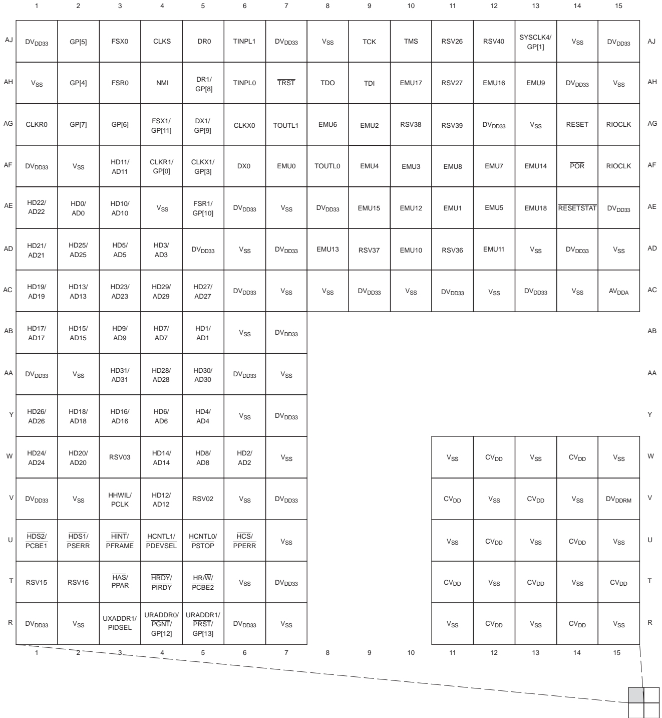
Figure 2-2. C6455 Pin Map (Bottom View) [Quadrant A]
