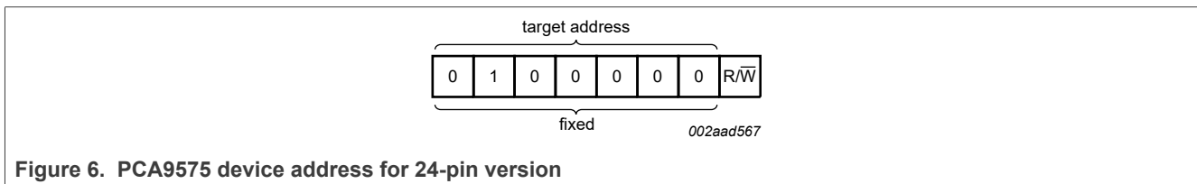
Figure 6. PCA9575 device address for 24-pin version
