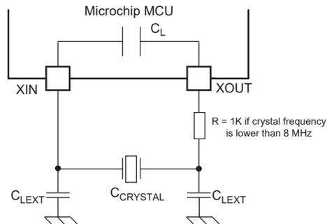
$$C_{LEXT} = 2 \times (C_{CRYSTAL} - C_L - C_{PCB})$$
