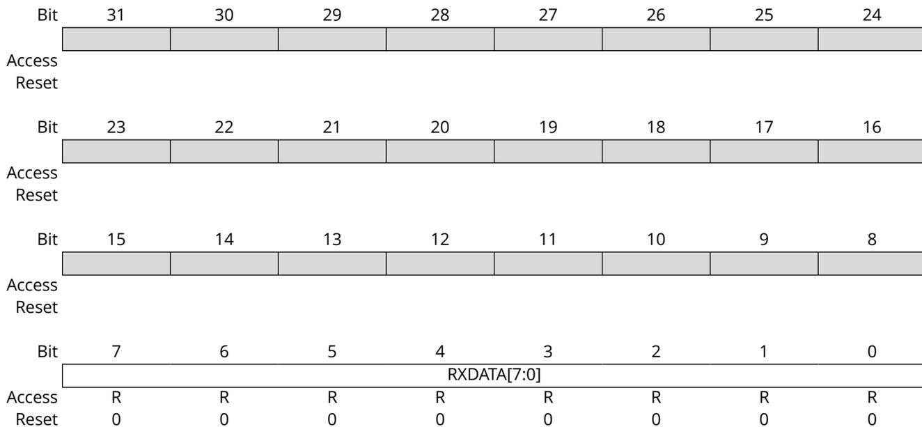
**Bits 7:0 – RXDATA[7:0]** Host or Client Receive Holding Data
