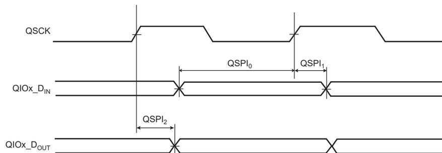
**Figure 57-18.** QSPI Host Mode with (CPOL = CPHA = 0) or (CPOL = CPHA = 1)
