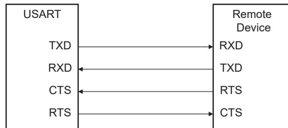
Setting the USART to operate with hardware handshaking is performed by writing the value 0x2 to US\_MR.USART\_MODE.
