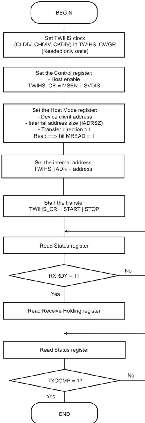
Figure 42-23. TWIHS Read Operation with Multiple Data Bytes with or without Internal Address
