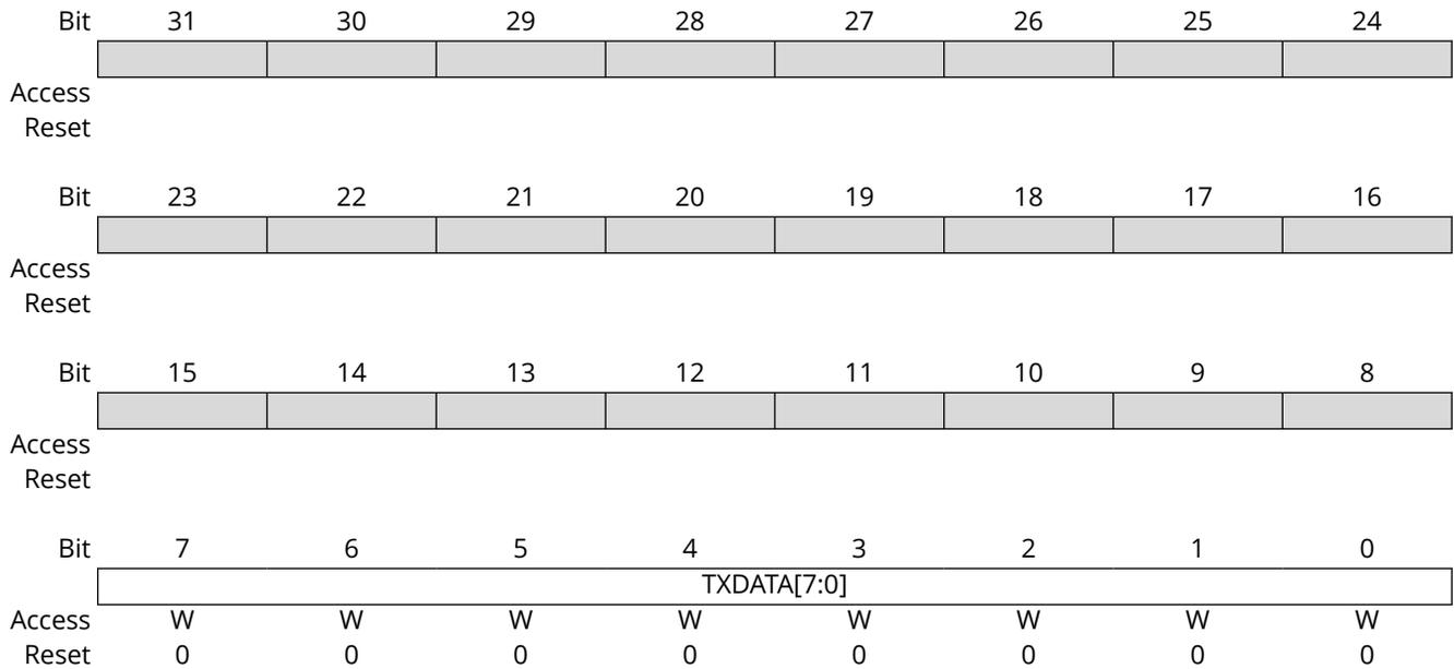
**Bits 7:0 - TXDATA[7:0]** Host or Client Transmit Holding Data
