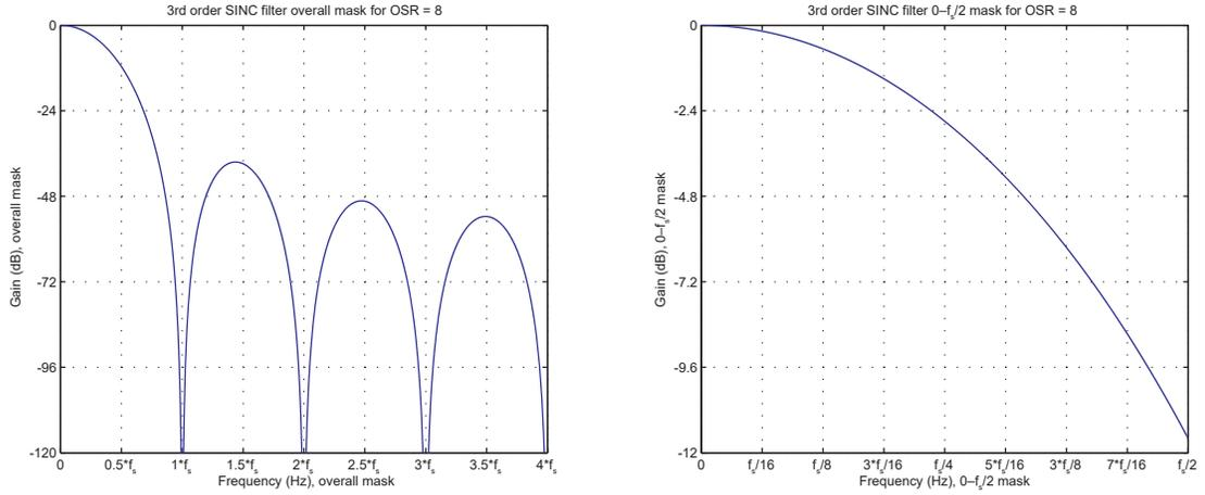
Figure 52-8. Interpolator Spectral Mask for OSR = 16
