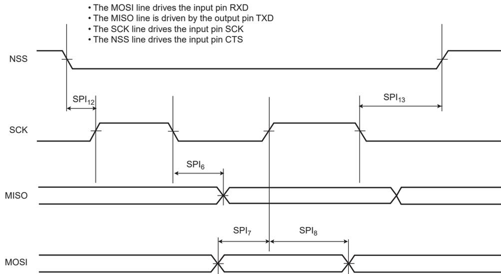
**Figure 57-28.** USART SPI Client Mode (Mode 0 or 3)
