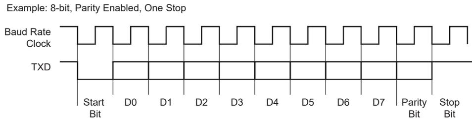
The characters are sent by writing in US\_THR. The transmitter reports two status bits in the Channel Status register (US\_CSR): TXRDY (Transmitter Ready), which indicates that US\_THR is empty, and TXEMPTY, which indicates that all the characters written in US\_THR have been processed. When the current character processing is completed, the last character written in US\_THR is transferred into the Shift register of the transmitter and US\_THR becomes empty, thus TXRDY rises.
