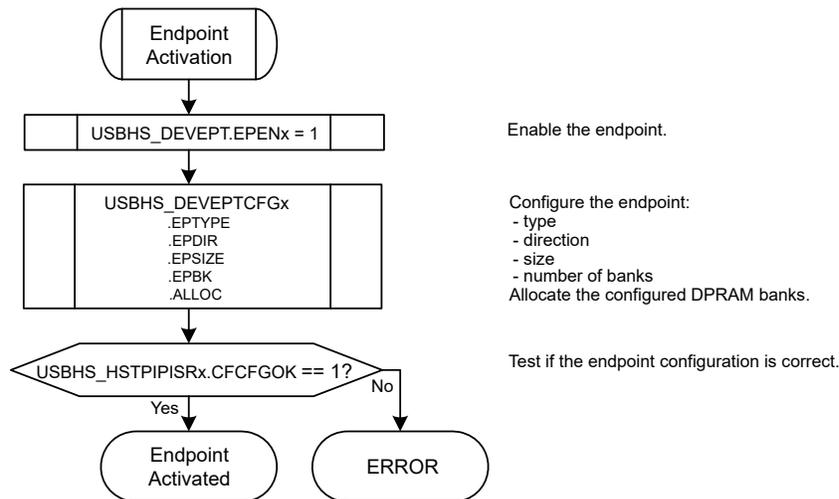
As long as the endpoint is not correctly configured (USBHS\_HSTPIISRx.CFGOK = 0), the controller does not acknowledge the packets sent by the host to this endpoint.
