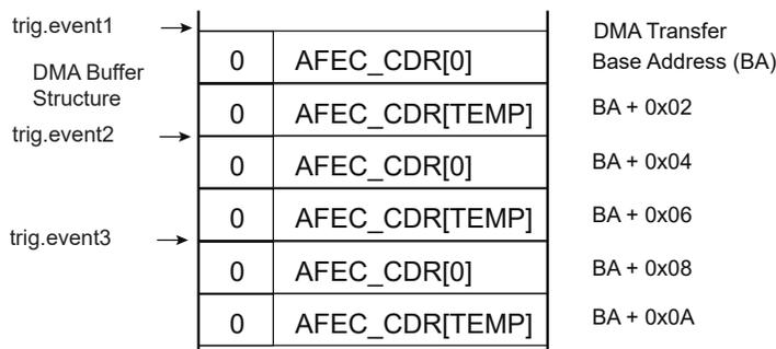
The temperature factor has a slow variation rate and may be different from other conversion channels. As a result, the AFEC allows a different way of triggering temperature measurement when AFEC\_TEMP\_MR.RTCT is set but AFEC\_CHSR.CH11 is cleared.
