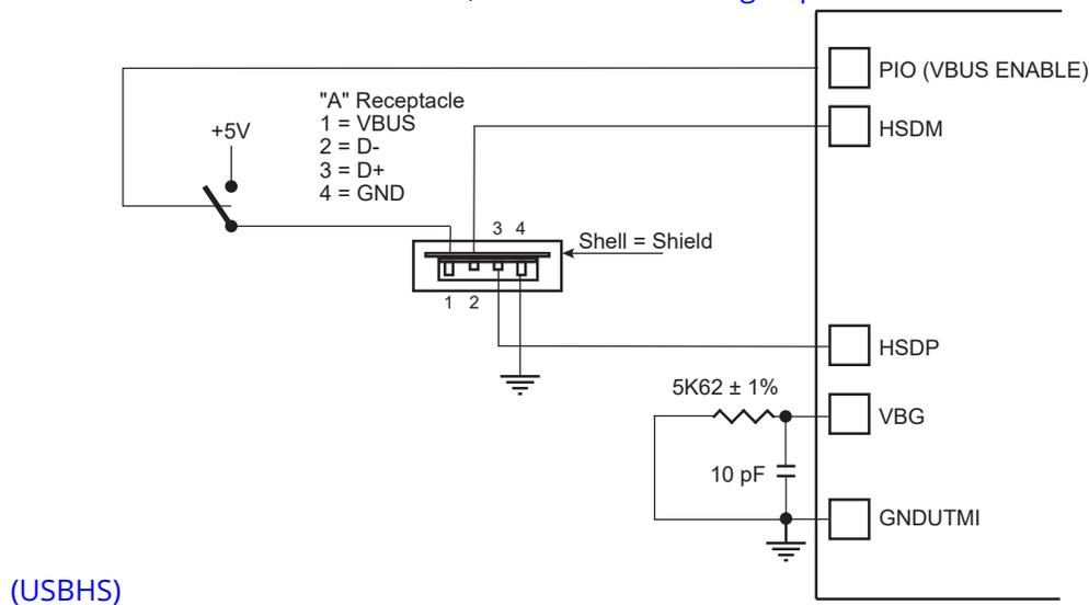
2. The following schematic shows a typical USB High Speed device connection: For more information, refer to [38. USB High-Speed Interface](#)
