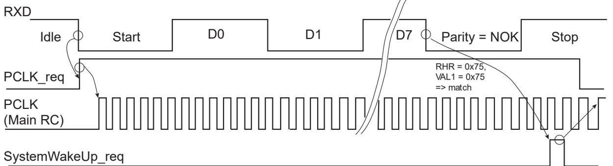
**Figure 46-13.** Asynchronous Event Generating Only Partial Wake-up
