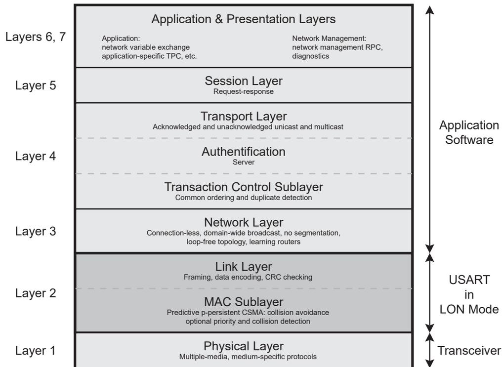
The USART configured in LON mode is a full-layer 2 implementation including standard timings handling, framing (transmit and receive PPDU frames), backlog estimation and other features. At the frame encoding/decoding level, differential Manchester encoding is used (also known as CDP). When configured in LON mode, there is no embedded digital line filter, thus the optimal usage is node-to-node communication.
