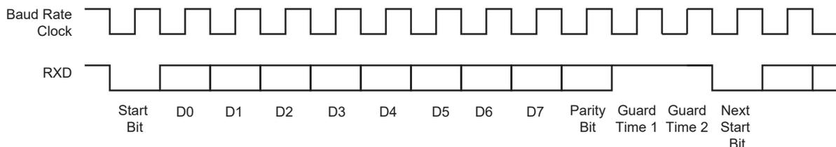
**Figure 45-31.** T = 0 Protocol with Parity Error
