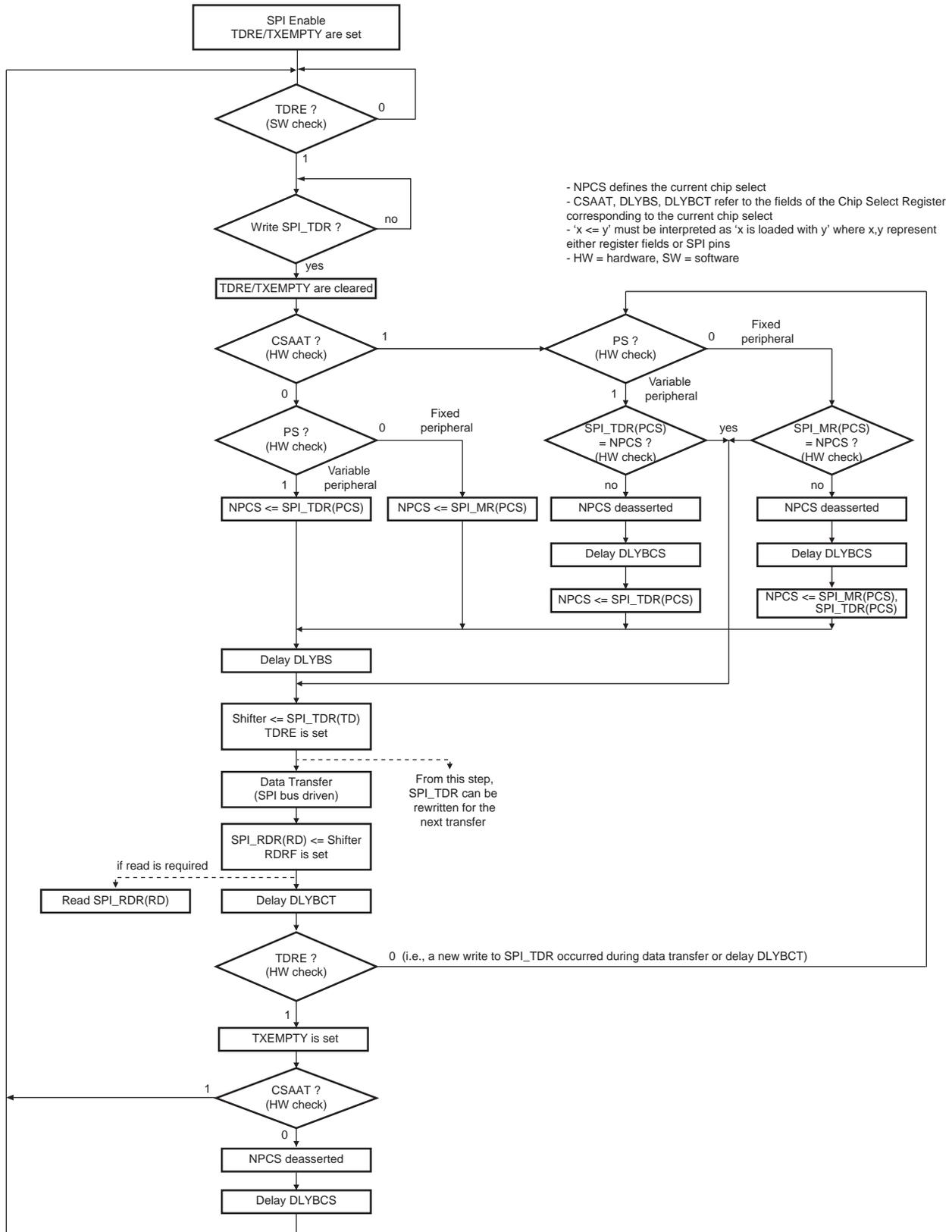
The figure below shows the behavior of Transmit Data Register Empty (TDRE), Receive Data Register (RDRF) and Transmission Register Empty (TXEMPTY) status flags within SPI\_SR during an 8-bit data transfer in Fixed mode without the DMA involved.
