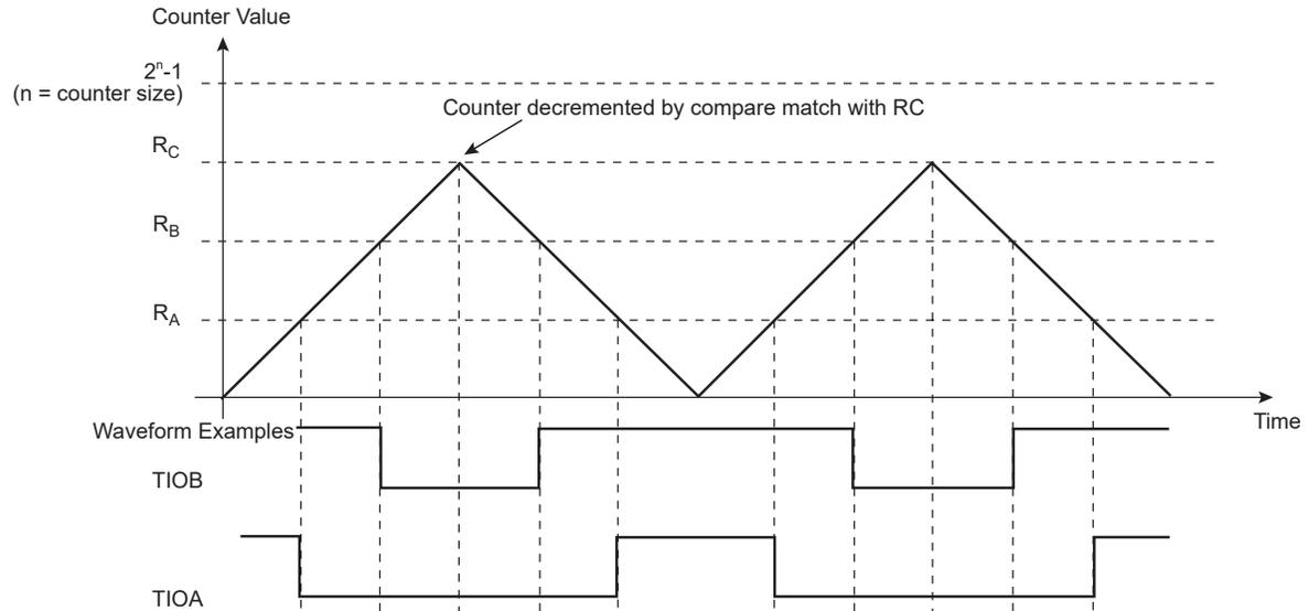
**Figure 49-15.** WAVSEL = 11 with Trigger
