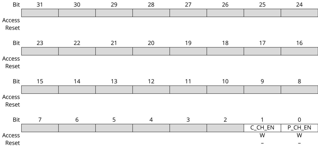
**Bit 1 - C\_CH\_EN** Codec Channel Enable
