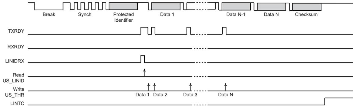
**Figure 45-49.** Client Node Configuration, NACT = SUBSCRIBE
