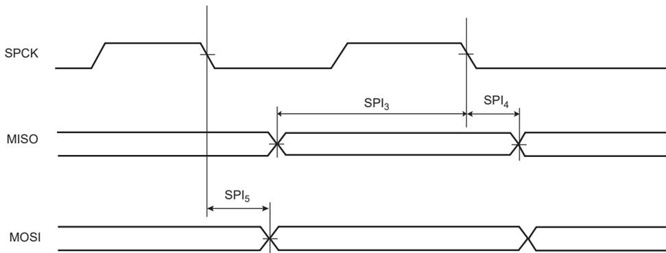
**Figure 57-22.** SPI Client Mode with (CPOL=0 and NCPHA=1) or (CPOL=1 and NCPHA=0)
