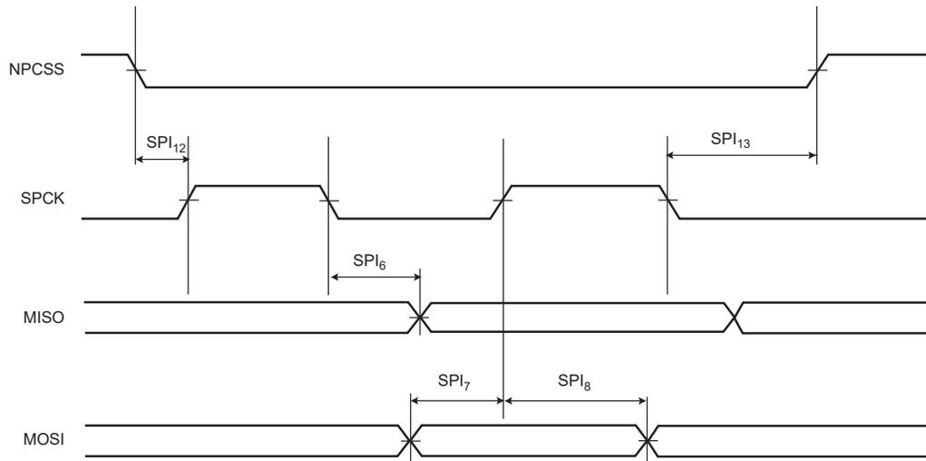
**Figure 58-23.** SPI Client Mode with (CPOL = NCPHA = 0) or (CPOL= NCPHA= 1)
