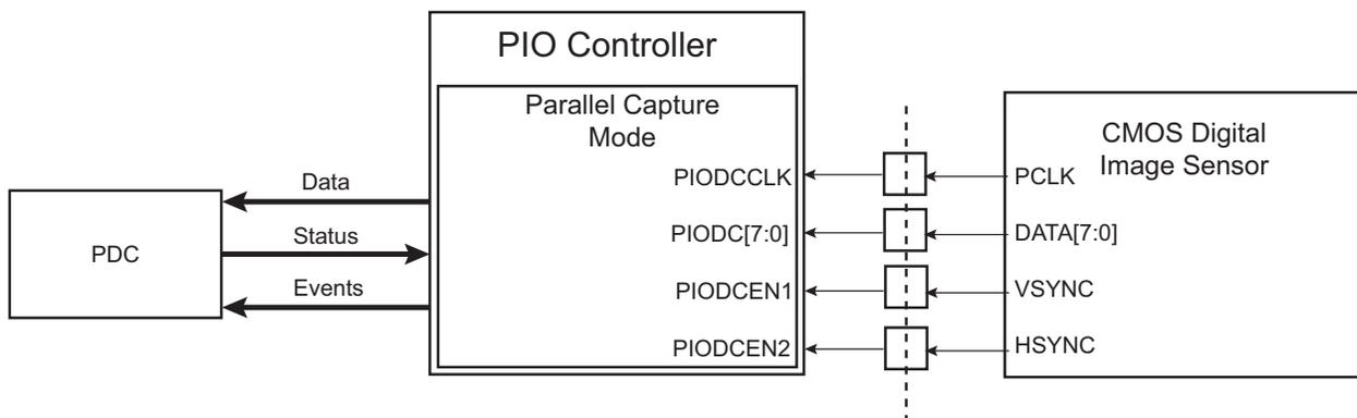
As soon as the Parallel Capture mode is enabled by writing a one to the PCEN bit in PIO\_PCMR, the I/O lines connected to the sensor clock (PIODCCLK), the sensor data (PIODC[7:0]) and the sensor data enable signals (PIODCEN1 and PIODCEN2) are configured automatically as inputs. To know which I/O lines are associated with the sensor clock, the sensor data and the sensor data enable signals, refer to the I/O multiplexing table(s) in the section “Package and Pinout”.
