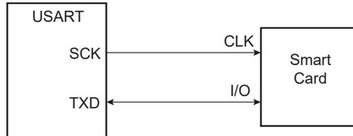
When operating in ISO7816, either in T = 0 or T = 1 modes, the character format is fixed. The configuration is 8 data bits and 1 or 2 stop bits, regardless of the values programmed in the Mode register fields CHRL, MODE9 and CHMODE. US\_MR.MSBF can be used to transmit LSB or MSB first. The bit INVDATA can be used to transmit in Normal or Inverse mode. See 45.7.3. US\_MR.
