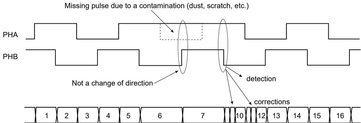
If a quadrature device is undamaged, the number of pulses counted for a predefined period of time must be the same with or without detection and autocorrection feature.
