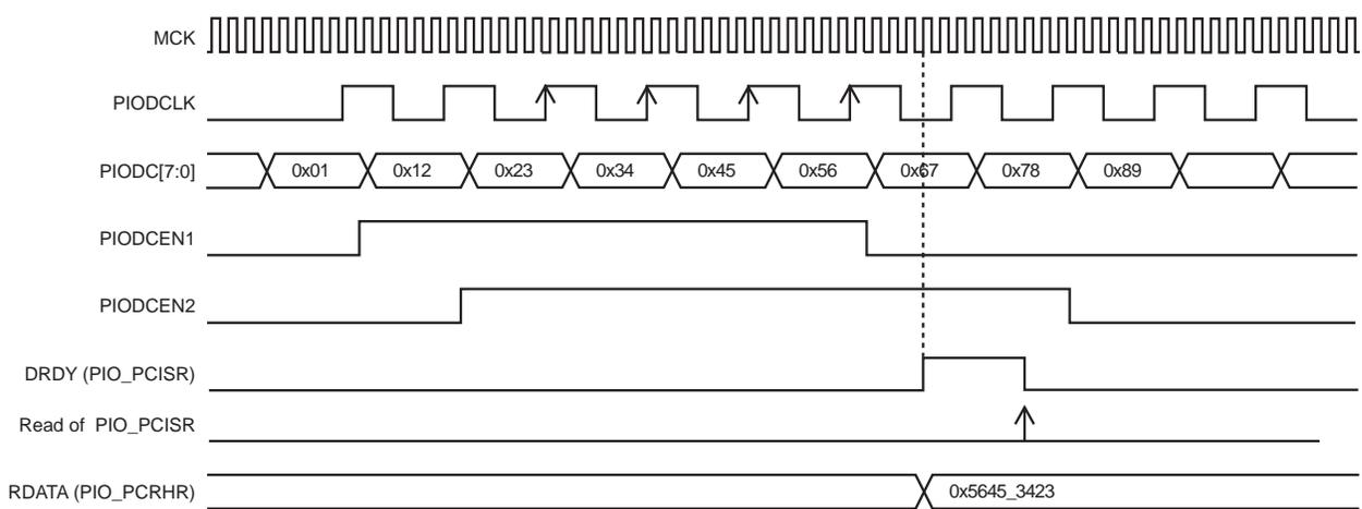
**Figure 32-11.** Parallel Capture Mode Waveforms (DSIZE = 2, ALWAYS = 1, HALFS = 0)
