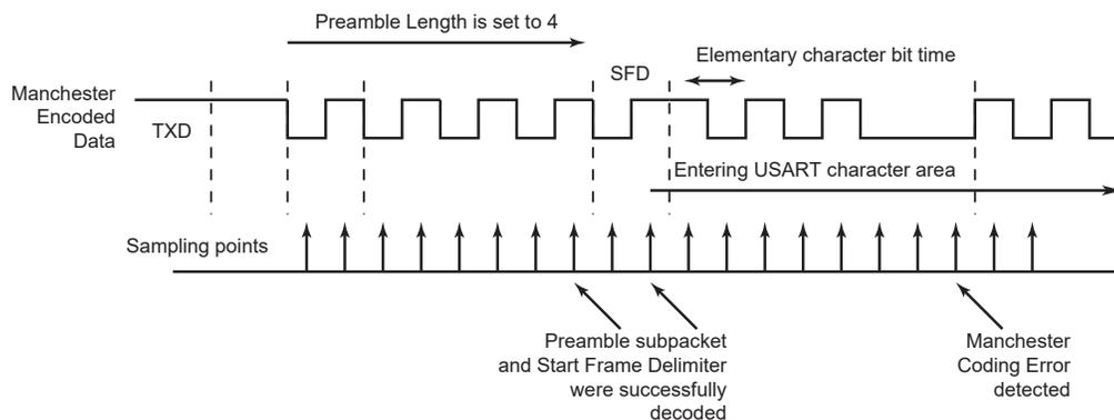
When the start frame delimiter is a sync pattern (US\_MR.ONEBIT = 0), both command and data delimiter are supported. If a valid sync is detected, the received character is written in RXCHR in the Receive Holding register (US\_RHR) and RXSYNH is updated. RXSYNH is set to '1' when the received character is a command, and to '0' if the received character is a data. This alleviates and simplifies the direct memory access as the character contains its own sync field in the same register.
