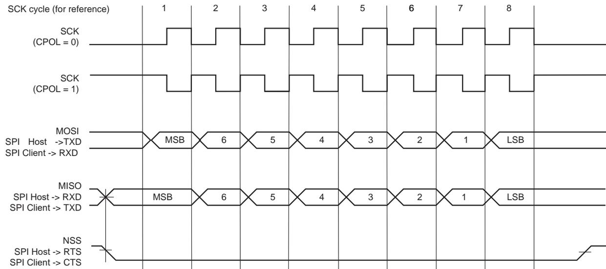
**Figure 45-38.** SPI Transfer Format (CPHA = 0, 8 bits per transfer)
