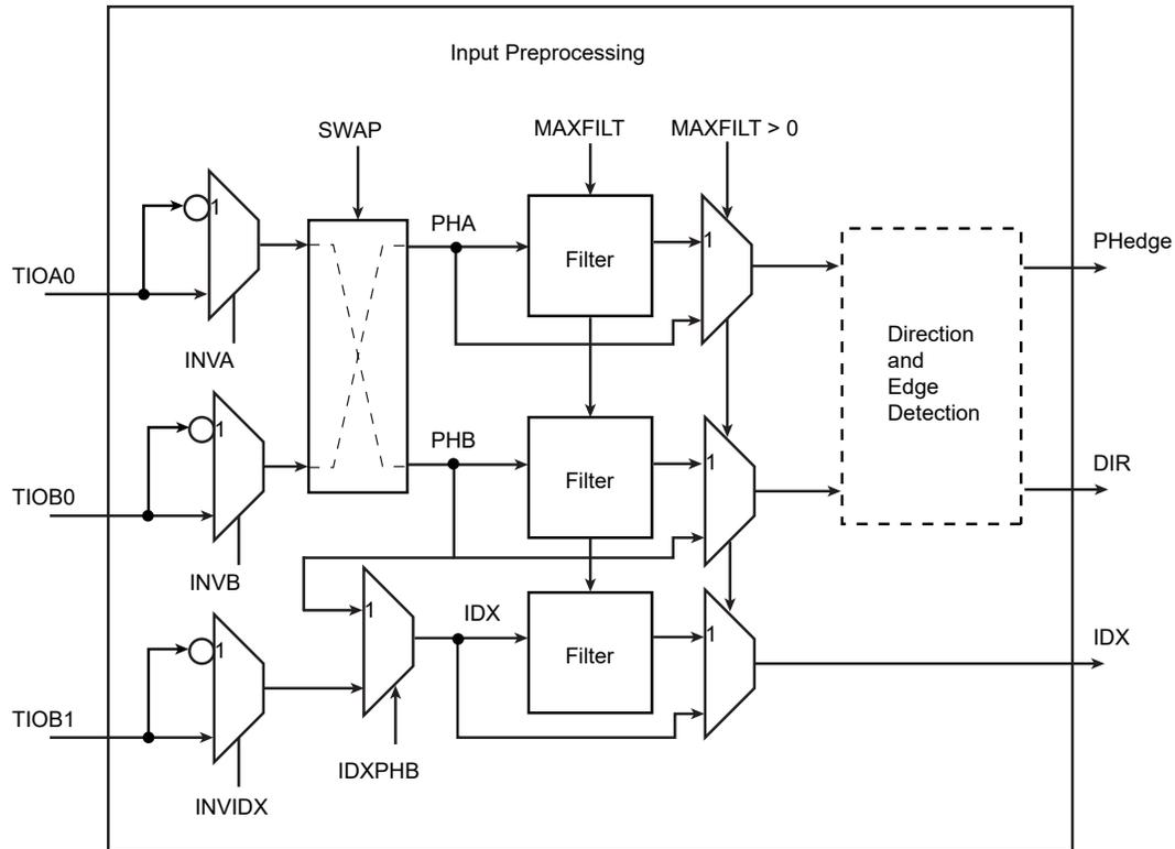
Input filtering can efficiently remove spurious pulses that might be generated by the presence of particulate contamination on the optical or magnetic disk of the rotary sensor.
