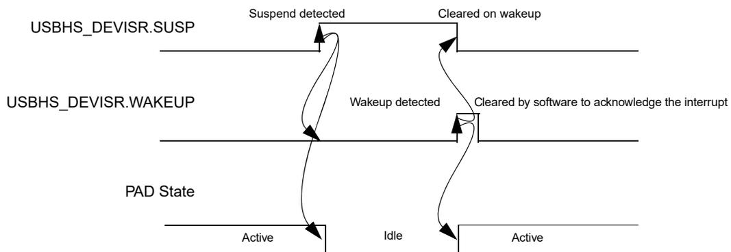
The USBHS\_DEVISR.SUSP bit is set and the Wakeup Interrupt (USBHS\_DEVISR.WAKEUP) bit is cleared when a USB "Suspend" state has been detected on the USB bus. This event automatically puts the USB pad in Idle state. The detection of a non-idle event sets USBHS\_DEVISR.WAKEUP, clears USBHS\_DEVISR.SUSP and wakes up the USB pad.
