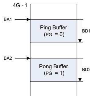
Each ADT entry holds a 32-bit BAn field which defines the start of each ping or pong buffer within system memory. The BDn field is used to indicate the size for the respective ping or pong page. The maximum size is 2k-entries for asynchronous and control channels; 8k-entries for isochronous and synchronous channels.
