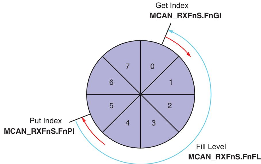
When reading from an Rx FIFO, Rx FIFO Get Index  $\text{MCAN\_RXFnS.FnGI} \times \text{FIFO Element Size}$  has to be added to the corresponding Rx FIFO start address  $\text{MCAN\_RXFnC.FnSA}$ .
