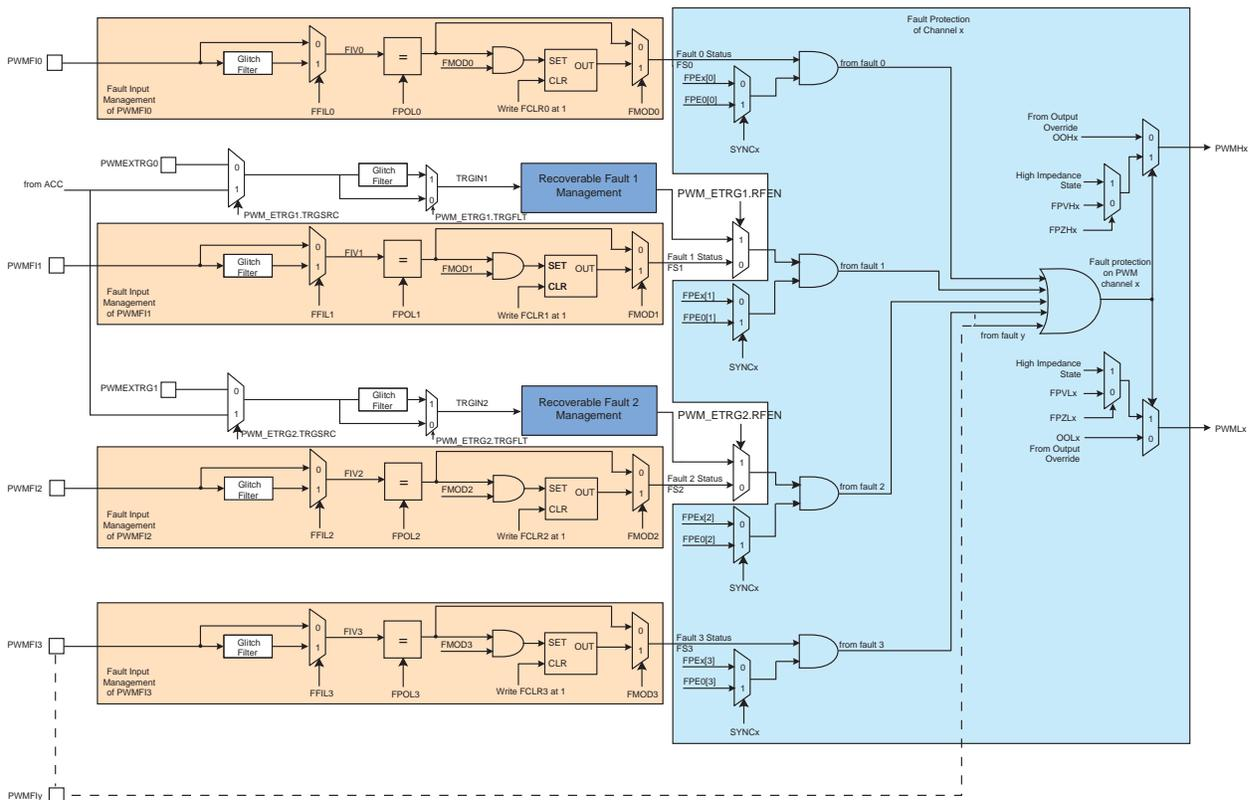
The polarity level of the fault inputs is configured by the FPOL field in the [PWM Fault Mode Register](#) (PWM\_FMR). For fault inputs coming from internal peripherals such as ADC or Timer Counter, the
