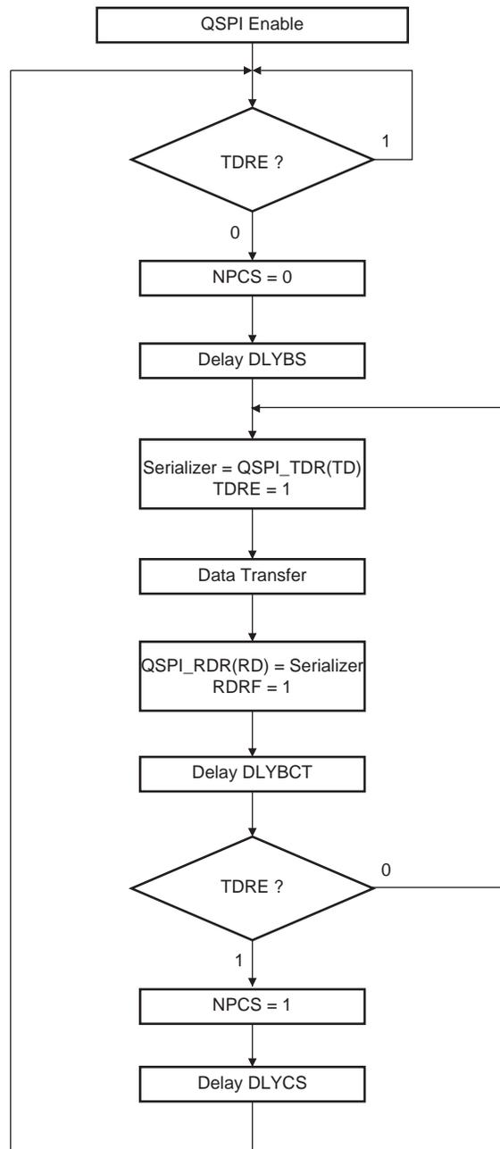
The figure below shows Transmit Data Register Empty (TDRE), Receive Data Register Full (RDRF) and Transmission Register Empty (TXEMPTY) status flags behavior within the QSPI\_SR during an 8-bit data transfer in Fixed mode, without DMA.
