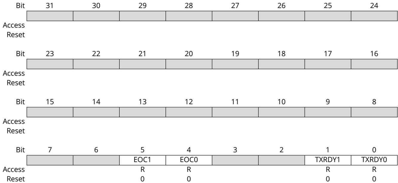
**Bits 4, 5 – EOCx** End of Conversion Interrupt Mask of channel x
