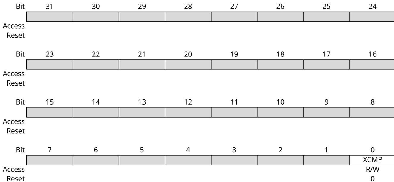
**Bit 0 - XCMP** Transfer Complete (Write 0 to Clear)
