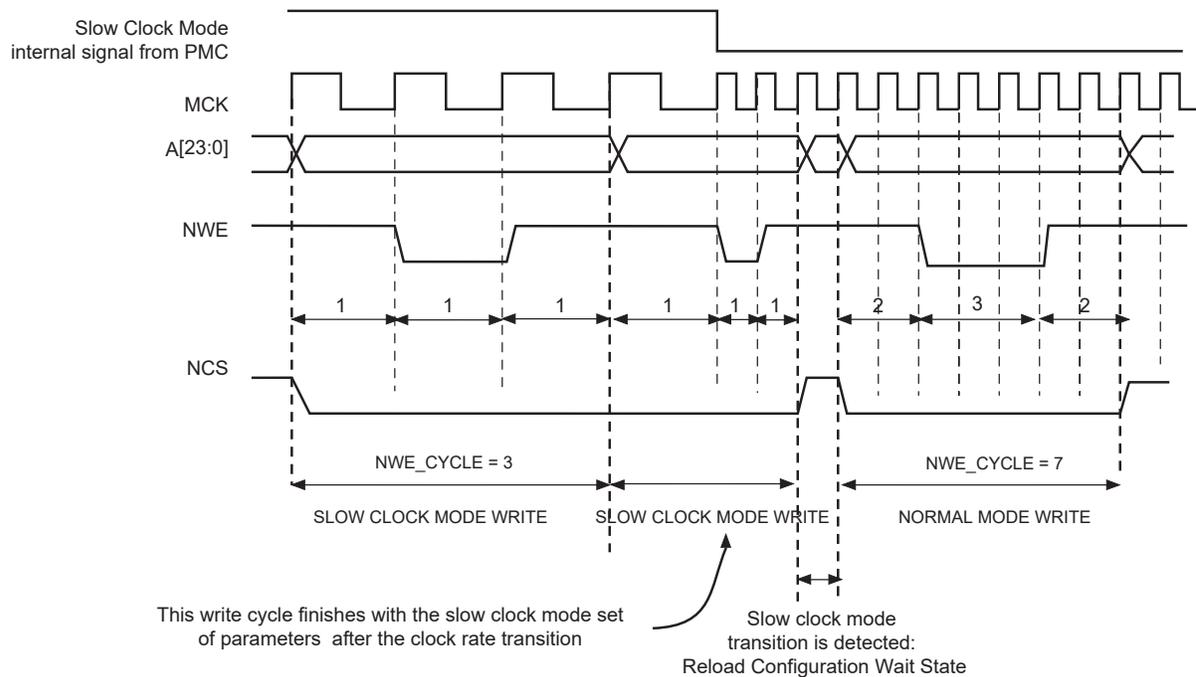
**Figure 34-34.** Recommended Procedure to Switch from Slow Clock Mode to Normal Mode or from Normal Mode to Slow Clock Mode
