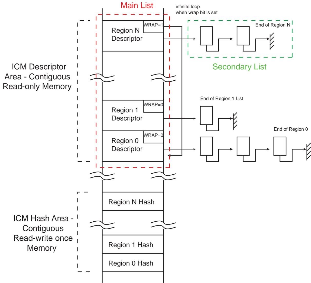
Each region descriptor supports gathering of data through the use of the Secondary List. Unlike the Main List, the Secondary List cannot modify the configuration attributes of the region. When the end of the Secondary List has been encountered, the ICM returns to the Main List. Memory integrity monitoring can be considered as a background service and the mandatory bandwidth shall be very limited. In order to limit the ICM memory bandwidth, use ICM\_CFG.BBC to control the ICM memory load.
