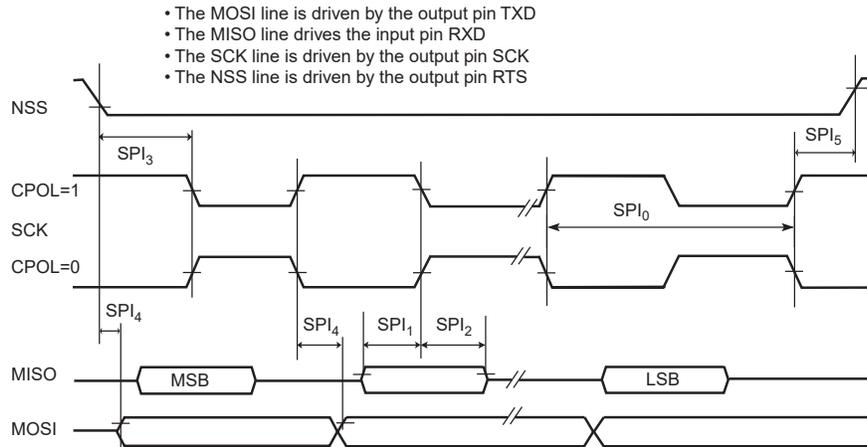
Figure 57-27. USART SPI Client Mode (Mode 1 or 2)
