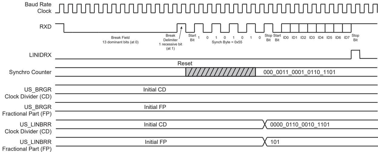
The accuracy of the synchronization depends on several parameters:
