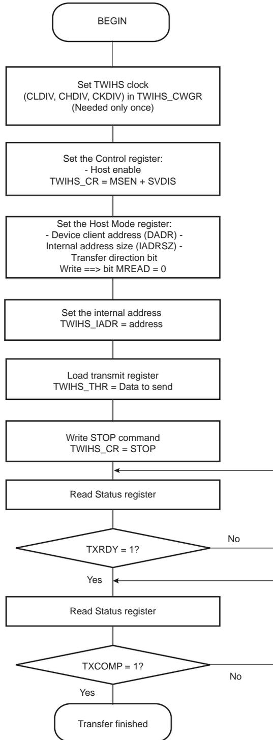
Figure 42-16. TWIHS Write Operation with Multiple Data Bytes with or without Internal Address
