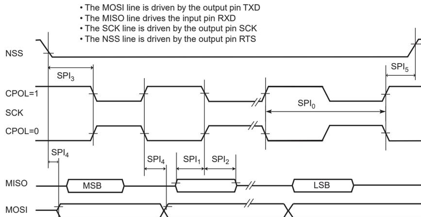
**Figure 58-25.** USART SPI Client Mode (Mode 1 or 2)
