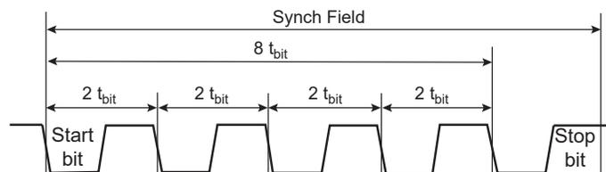
The time measurement is made by a 19-bit counter clocked by the sampling clock (see “Baud Rate Generator”).
