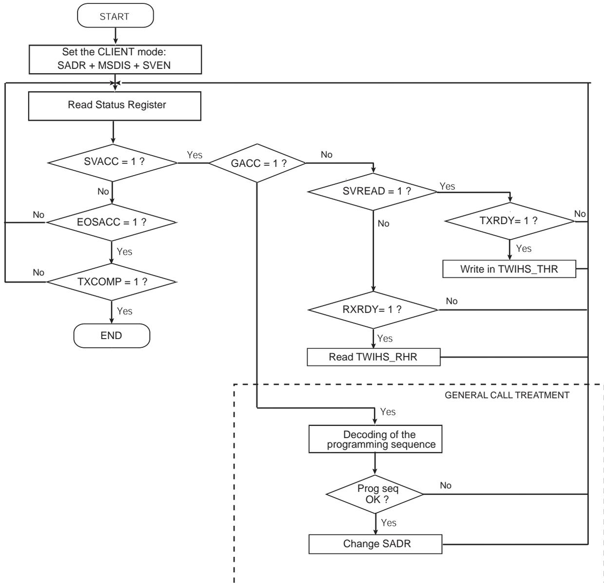
Figure 42-44. Read Write Flowchart in Client Mode with SMBus PEC
