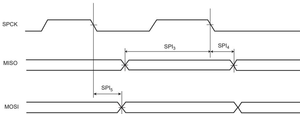
**Figure 58-22.** SPI Client Mode with (CPOL=0 and NCPHA=1) or (CPOL=1 and NCPHA=0)
