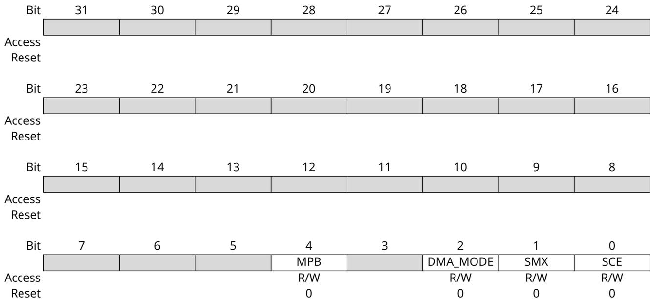
**Bit 4 - MPB** DMA Packet Buffering Mode
