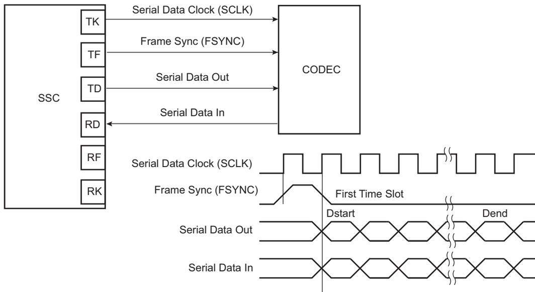
Figure 43-5. Time Slot Application Block Diagram
