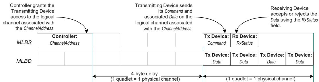
During normal operation, the MediaLB Controller initiates a transfer by sending out the ChannelAddress on the MLBS line, and then stops driving (high-impedance) the MLBS line. When a MediaLB Device recognizes the ChannelAddress as related to one of its channels, the Tx Device will generate the Command on the MLBS line and place the data on the MLBD line. The Rx Device will generate the RxStatus on the MLBS line, after the Command. Both Command and RxStatus
