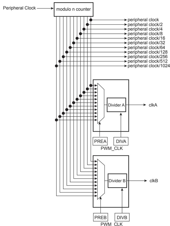
The PWM peripheral clock is divided in the clock generator module to provide different clocks available for all channels. Each channel can independently select one of the divided clocks.
