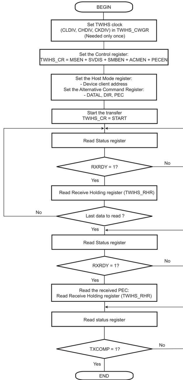
Figure 42-26. TWIHS Read Operation with Multiple Data Bytes + Write Operation with Multiple Data Bytes (Sr)
