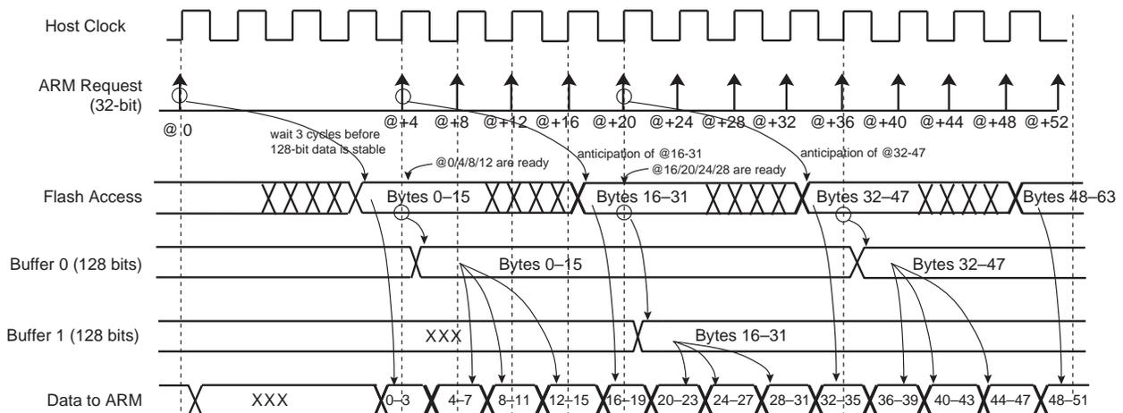
**Note:** When FWS is between 1 and 3, in case of sequential reads, the first access takes (FWS + 1) cycles. The following accesses take only one cycle.
