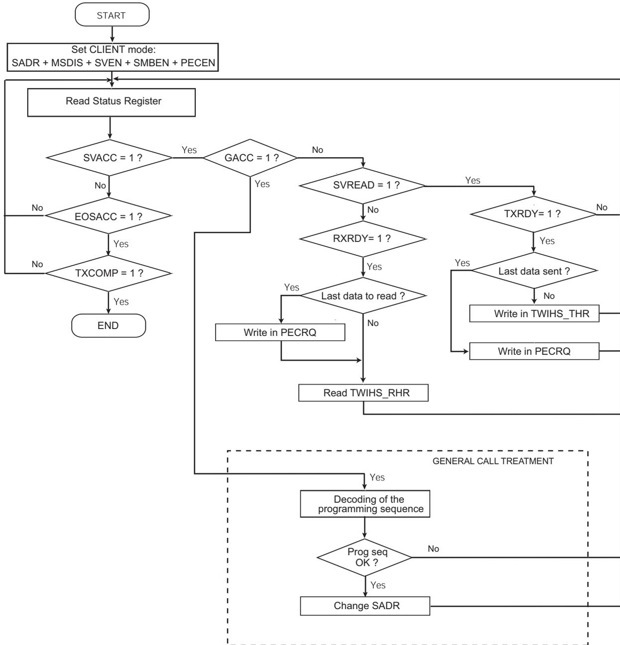
Figure 42-45. Read Write Flowchart in Client Mode with SMBus PEC and Alternative Command Mode
