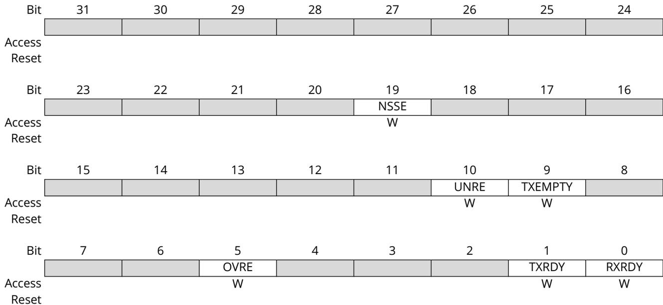
**Bit 19 – NSSE** NSS Line (Driving CTS Pin) Rising or Falling Edge Event Interrupt Disable
