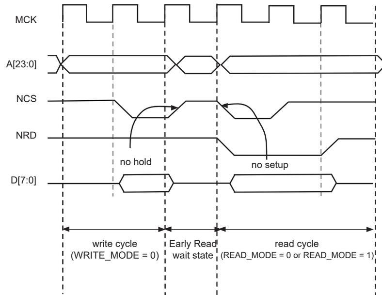
**Figure 34-20. Early Read Wait State: NWE-controlled write with no hold followed by a read with one set-up cycle**
