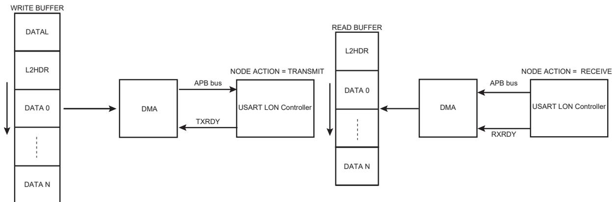
**Figure 45-64. DMAM = 0**
