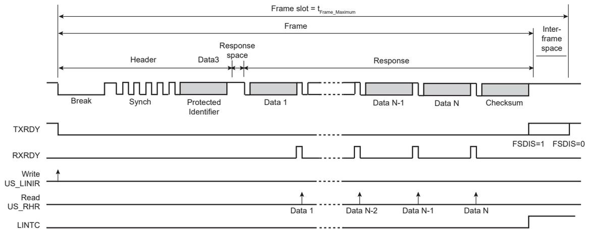
**Figure 45-47.** Host Node Configuration, NACT = IGNORE
