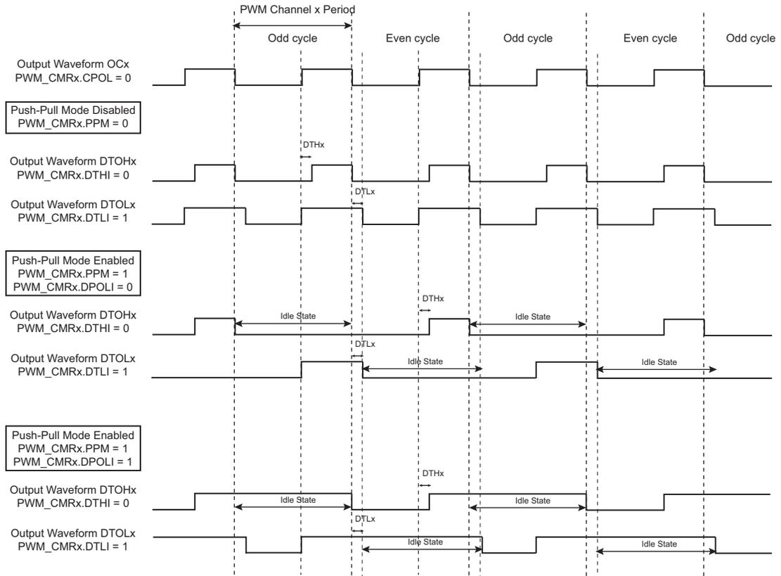
Figure 50-11. PWM Push-Pull Waveforms: Left-Aligned Mode
