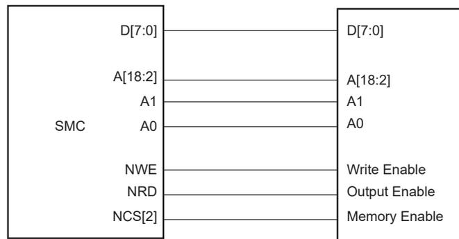
**Figure 34-3.** Memory Connection for a 16-bit Data Bus
