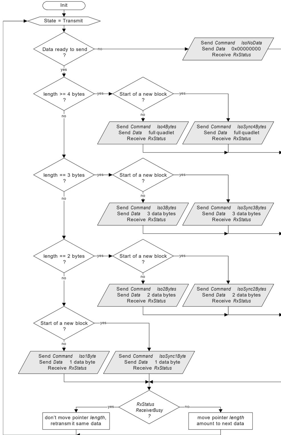
Figure 47-15. Isochronous Data Rx Device Protocol
