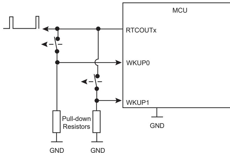
The debouncing period duration is configurable. The period is set for all debouncers (i.e., the duration cannot be adjusted for each debouncer). The number of successive identical samples to wake up the system can be configured from 2 up to 8 in SUPC\_WUMR.LPDBC. The period of time between two samples can be configured by programming RTC\_MR.TPERIOD. Power parameters can be adjusted by modifying the period of time in RTC\_MR.THIGH.
