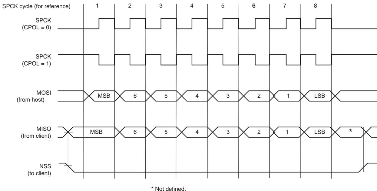
**Figure 40-4.** SPI Transfer Format (NCPHA = 0, 8 bits per transfer)
