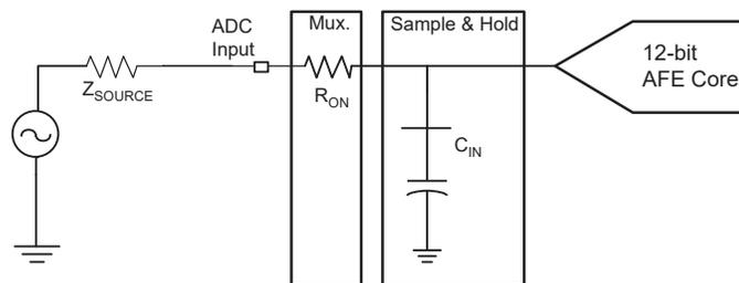
During the tracking phase, the AFE tracks the input signal during the tracking time shown below:
