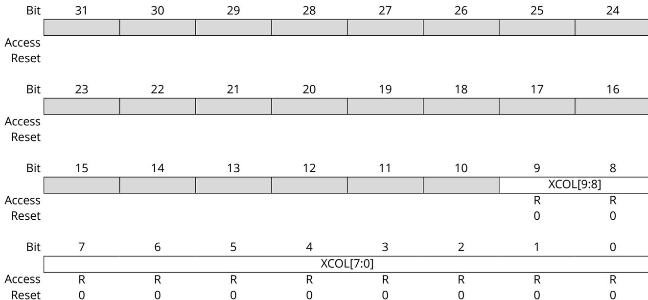
**Bits 9:0 – XCOL[9:0]** Excessive Collisions
