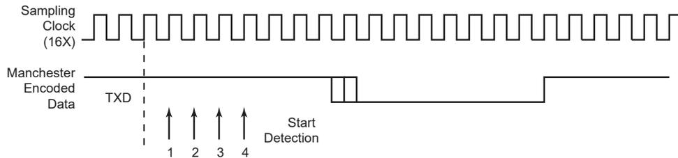
The receiver is activated and starts preamble and frame delimiter detection, sampling the data at one quarter and then three quarters. If a valid preamble pattern or start frame delimiter is detected, the receiver continues decoding with the same synchronization. If the stream does not match a valid pattern or a valid start frame delimiter, the receiver resynchronizes on the next valid edge. The minimum time threshold to estimate the bit value is three quarters of a bit time.
