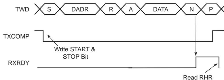
**Figure 42-8. Host Read with Multiple Data Bytes**
