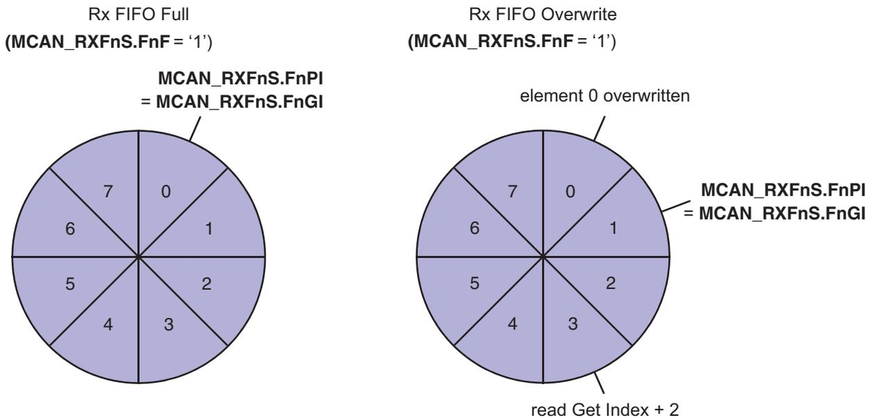
After reading from the Rx FIFO, the number of the last element read has to be written to the Rx FIFO Acknowledge Index `MCAN_RXFnA.FnA`. This increments the get index to that element number. In case the put index has not been incremented to this Rx FIFO element, the Rx FIFO full condition is reset (`MCAN_RXFnS.FnF = '0'`).
