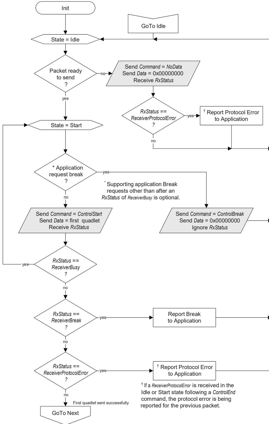
Figure 47-7. Control Packet Tx Device Protocol: Middle
