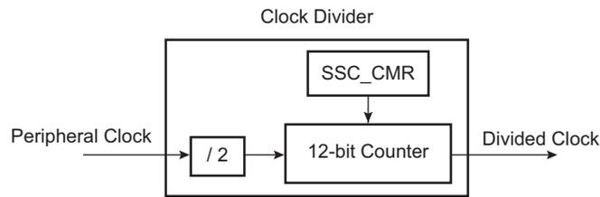
The peripheral clock divider is determined by the 12-bit field DIV counter and comparator (so its maximal value is 4095) in the Clock Mode Register (SSC\_CMCR), allowing a peripheral clock division by up to 8190. The Divided Clock is provided to both the receiver and the transmitter. When this field is programmed to 0, the Clock Divider is not used and remains inactive.
