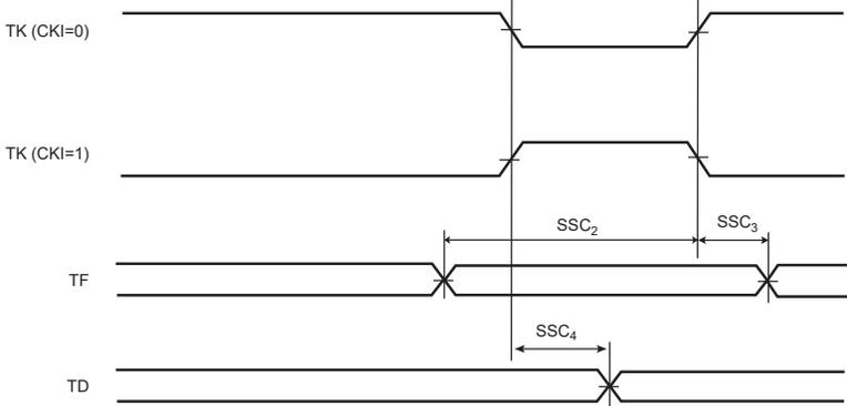
**Figure 58-34.** SSC Transmitter, TK and TF in Input
