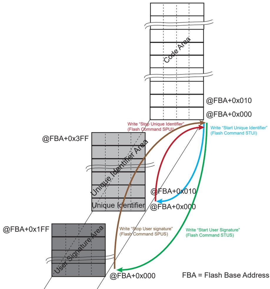
**Figure 22-2.** Organization of Embedded Flash for Code
