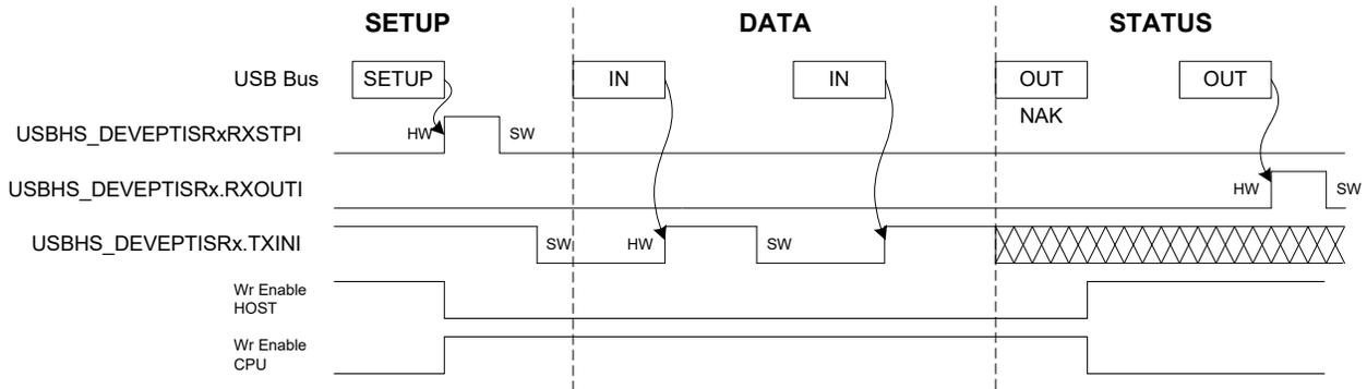
A NAK handshake is always generated on the first status stage command.
