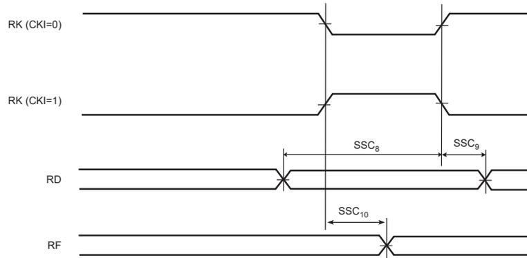
Figure 58-37. SSC Receiver, RK and RF in Output
