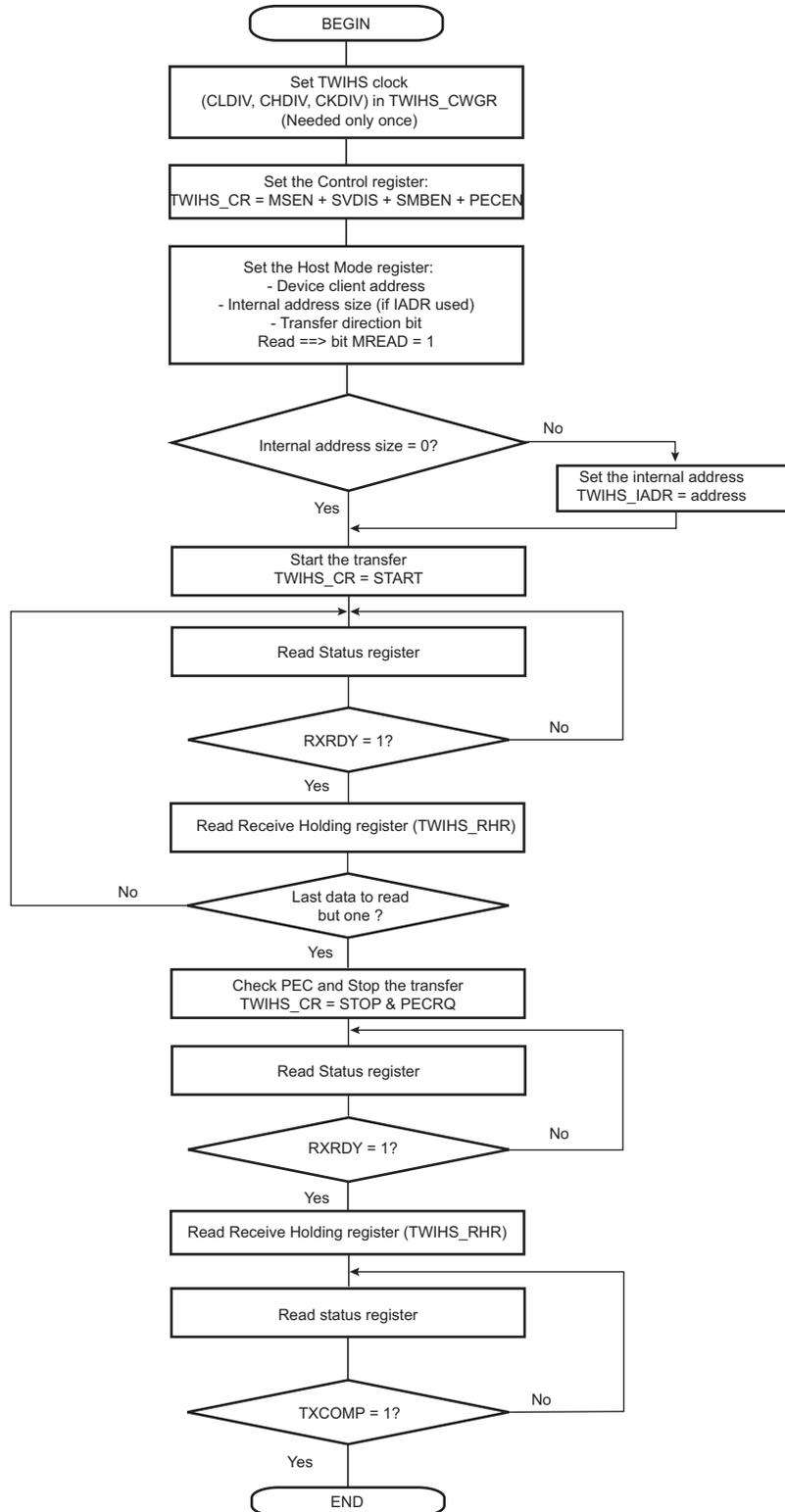
Figure 42-25. TWIHS Read Operation with Multiple Data Bytes with Alternative Command Mode with PEC
