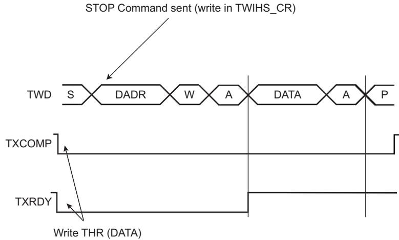
**Figure 42-5. Host Write with Multiple Data Bytes**
