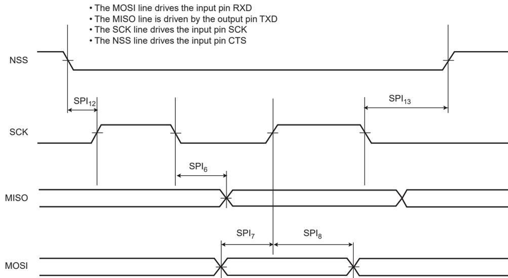
**Figure 58-26.** USART SPI Client Mode (Mode 0 or 3)
