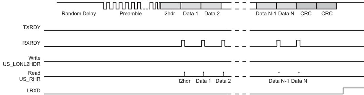
**45.6.10.12 LON Frame Handling with the Peripheral DMA Controller**
