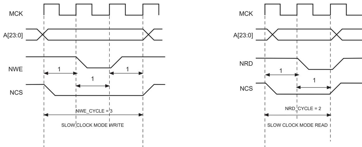
**Table 34-6.** Read and Write Timing Parameters in Slow Clock Mode
