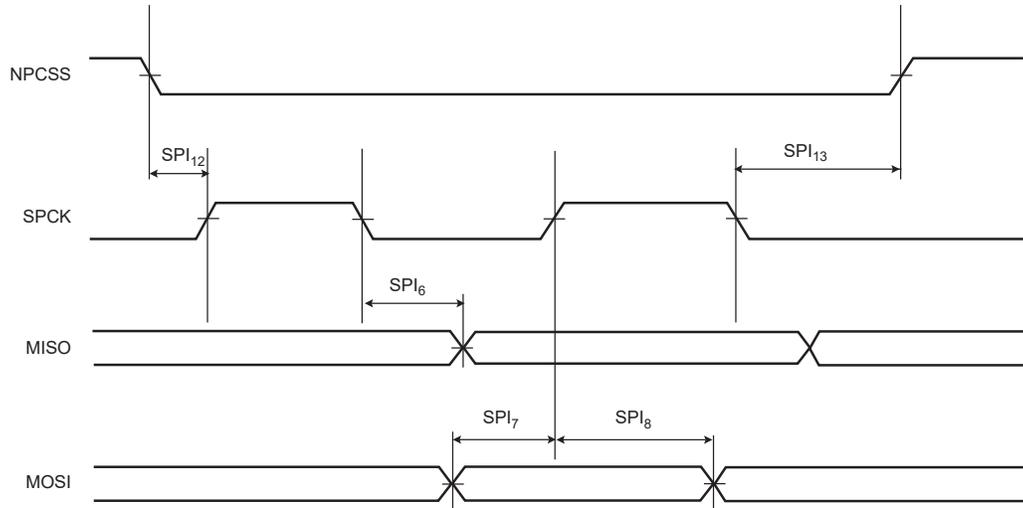
**Figure 57-23.** SPI Client Mode with (CPOL = NCPHA = 0) or (CPOL= NCPHA= 1)
