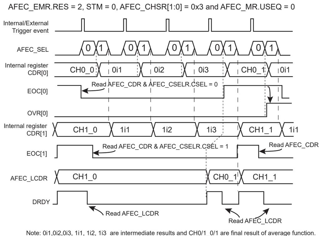
If AFEC\_EMR.STM is set and AFEC\_MR.USEQ is cleared, the sequence to be converted, defined in the AFEC\_CHSR, is automatically repeated n times, where n corresponds to the oversampling ratio defined AFEC\_EMR.RES. As a result, only one trigger is required to get the result of the averaging function as shown in the figure below.
