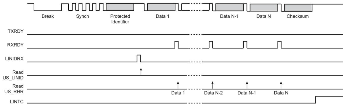
**Figure 45-50.** Client Node Configuration, NACT = IGNORE
