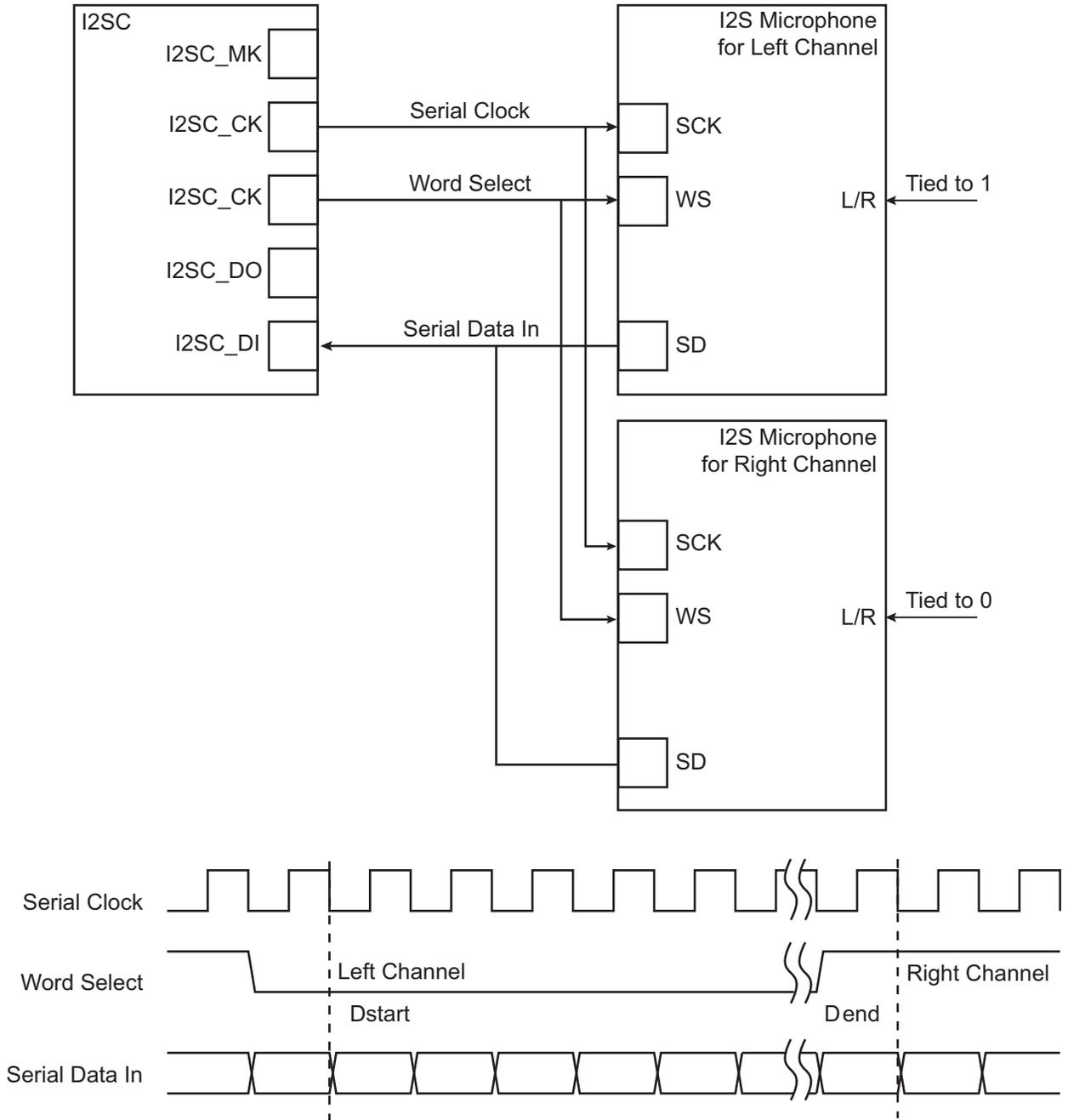
Figure 44-7. Codec Application Block Diagram
