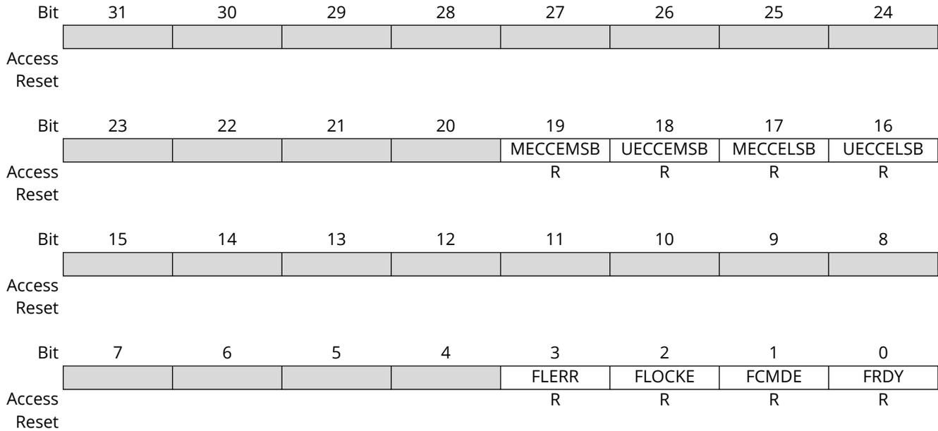
**Bit 19 – MECC EMSB** Multiple ECC Error on MSB Part of the Memory Flash Data Bus (cleared on read)
