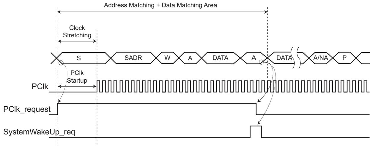
**Figure 42-42. Address Match and No Data Match (Data Matching Enabled)**
