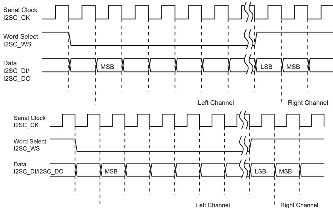
Data bits are sent on the falling edge of the serial clock and sampled on the rising edge of the serial clock. The word select line indicates the channel in transmission, a low level for the left channel and a high level for the right channel.
