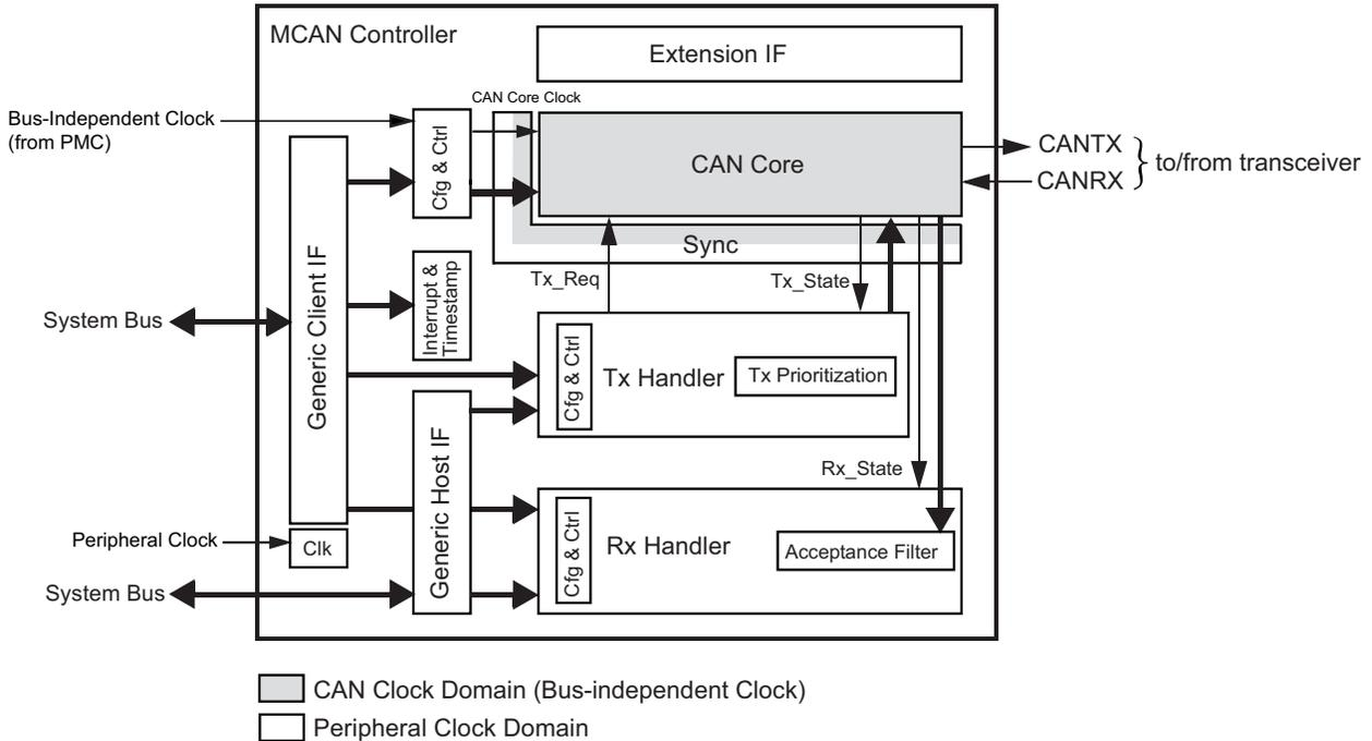
**Note:** Refer to section “Power Management Controller (PMC)” for details about the bus-independent clock (PCK5).
