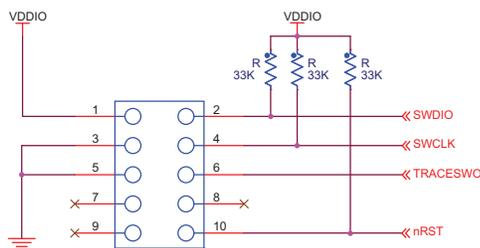
Figure 59-2. SWD Schematic Example with a 20-pin Connector
