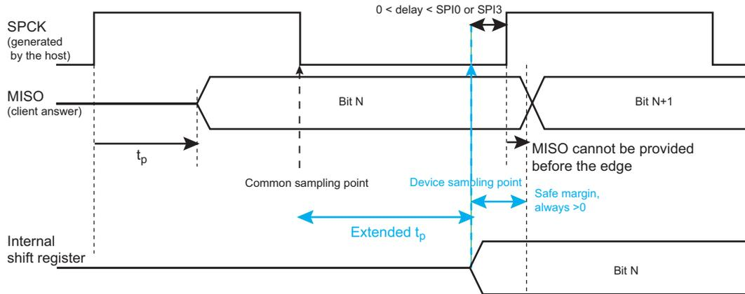
**Figure 57-20.** SPI Host Mode with (CPOL= NCPHA = 0) or (CPOL= NCPHA= 1)
