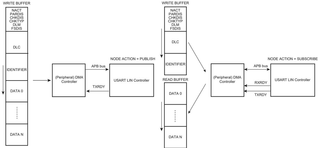
**Figure 45-52.** Host Node with DMAC (PDCM = 0)
