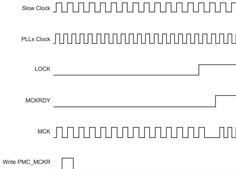
**Figure 31-7.** Switch Host Clock (MCK) from Main Clock (MAINCK) to Slow Clock
