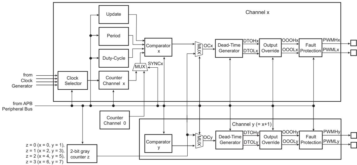
Each of the 4 channels is composed of six blocks:
