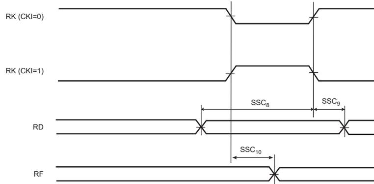
Figure 57-39. SSC Receiver, RK and RF in Output
