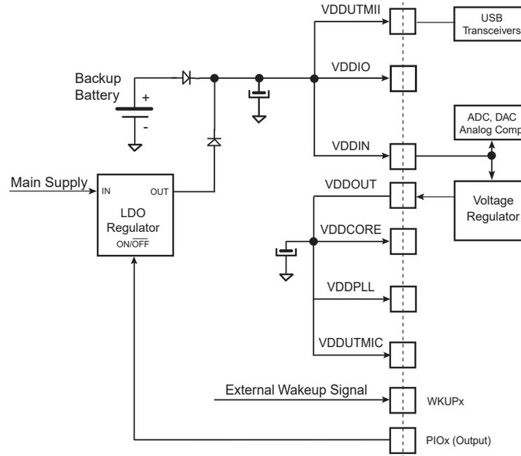
Note: The two diodes provide a "switchover circuit" between the backup battery and the main supply when the system is put in Backup mode.
