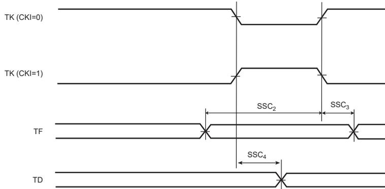
**Figure 57-36. SSC Transmitter, TK and TF in Input**
