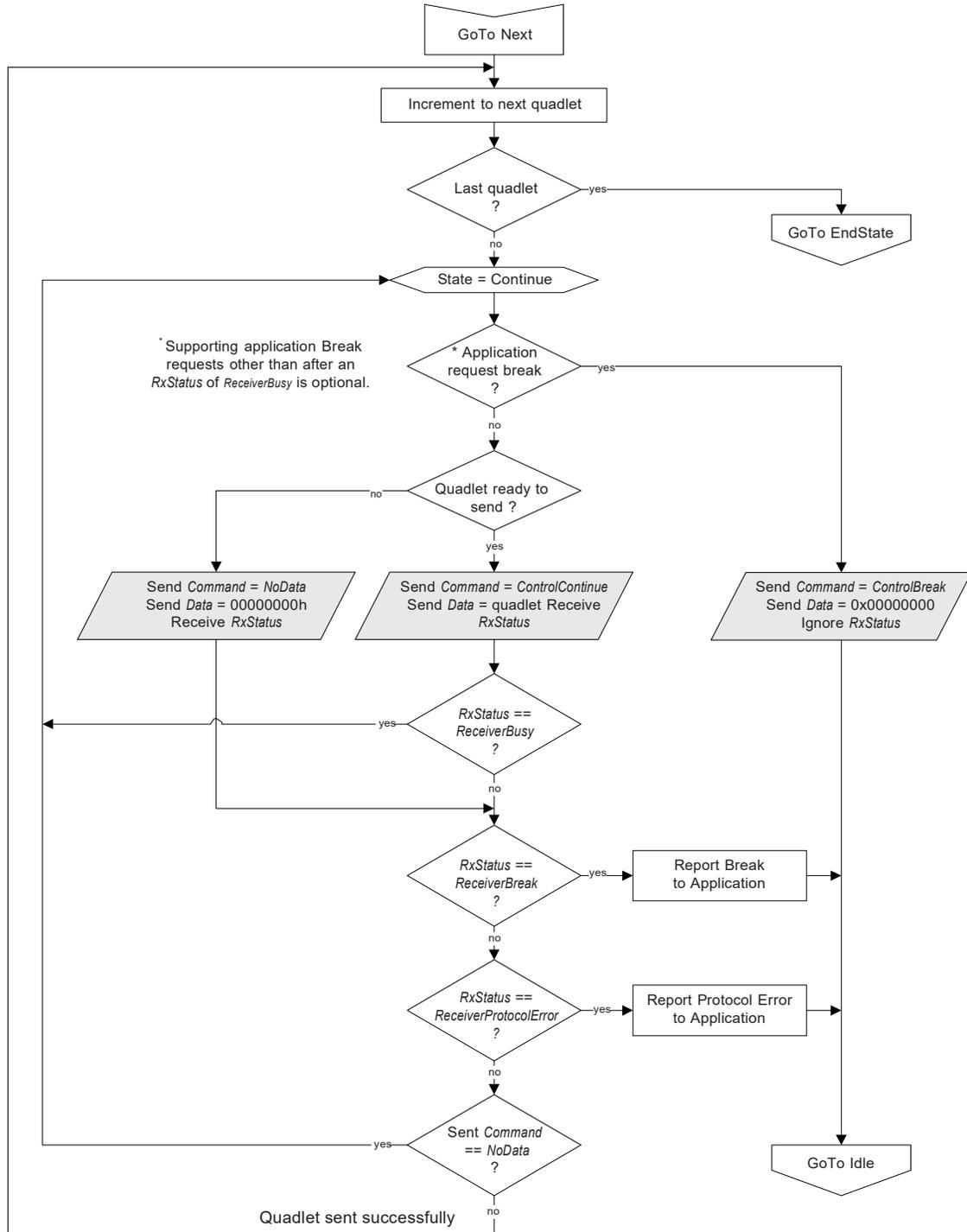
Figure 47-8. Control Packet Tx Device Protocol: End
