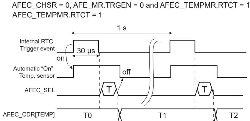
Moreover, it is possible to raise a flag only if there is predefined change in the temperature measurement. The user can define a range of temperature or a threshold in AFEC\_TEMPMPR and the mode of comparison in AFEC\_TEMPMPR. These values define the way the TEMPCHG flag will be raised in AFEC\_ISR.
