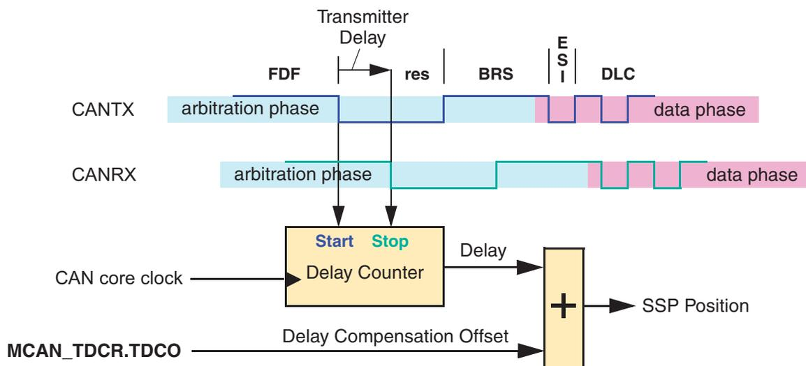
To avoid that a dominant glitch inside the received FDF bit ends the delay compensation measurement before the falling edge of the received res bit, resulting in a too early SSP position,
