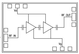
odes to limit the applied voltage. Also, make sure to sequence the applied voltage to ensure negative gate bias is available before applying the positive drain supply.
