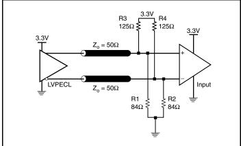
Figure 3B. 3.3V LVPECL Output Termination
