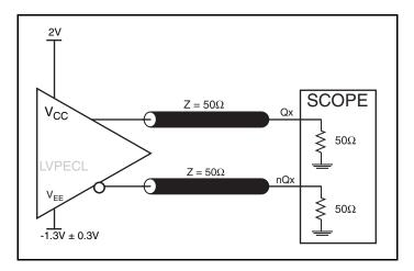
LVPECL Output Load AC Test Circuit
