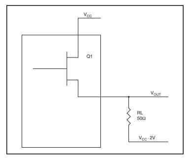
Figure 4. LVPECL Driver Circuit and Termination
