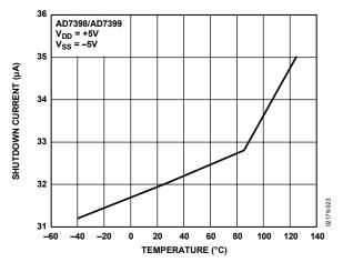
Figure 23. Shutdown Current vs. Temperature
