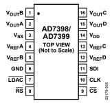
Figure 5. Pin Configuration
