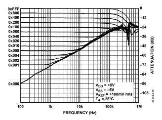
Figure 19. AD7398 Multiplying Gain vs. Frequency
