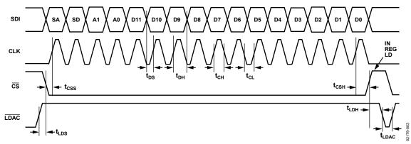
Figure 3. AD7398 Timing Diagram (AD7399 with SDI = 14 Bits Only)
