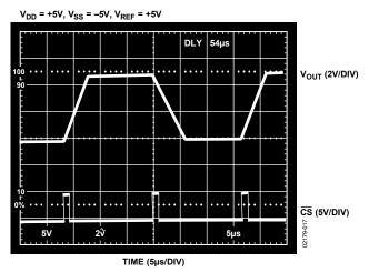
Figure 17. AD7398 Large Signal Settling Time
