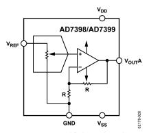
Figure 26. Simplified DAC Channel
