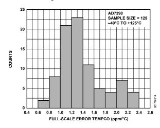
Figure 14. AD7398 Full-Scale Error Tempco
