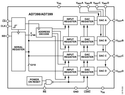
Figure 25. Simplified Block Diagram
