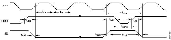
Figure 4. Continuous Clock Timing Diagram
