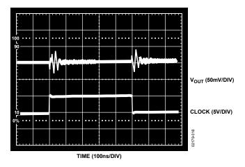
Figure 16. AD7398 Digital Feedthrough
