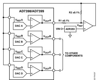
Figure 37. Programmable DAC Reference
