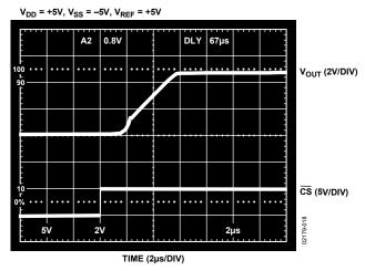
Figure 18. AD7398 Shutdown Recovery
