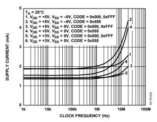
Figure 20. AD7398 Supply Current vs. Clock Frequency
