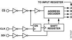
Figure 27. Equivalent Logic Interface
