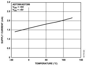
Figure 22. Supply Current vs. Temperature
