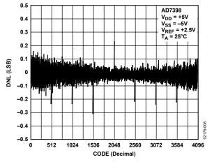
Figure 8. AD7398 DNL vs. Code ( $T_A = 25$  °C)
