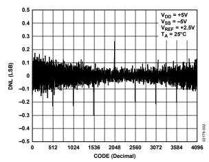
Figure 2. AD7398 DNL vs. Code ( $T_A = 25$ °C)
