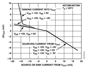
Figure 13. ΔV<sub>OUT</sub> vs. Load Current
