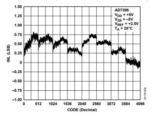
Figure 6. AD7398 INL vs. Code ( $T_A = 25$ °C)
