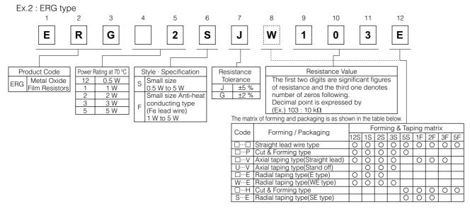
The above example 2 shows a small metal oxide film resistor, 2 W power rating, resistance value of 10  $k\Omega$ , tolerance  $\pm 5$  %, and package of radial taping.
