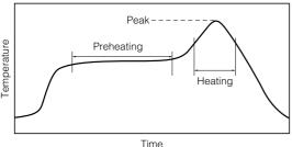
For soldering (Example: Sn-37Pb)
