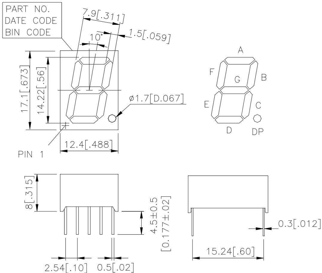
NOTES: All dimensions are in millimeters. Tolerances are  $\pm 0.25\text{mm}$  (0.01") unless otherwise noted.
