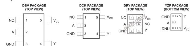
See mechanical drawings for dimensions. DNU - Do not use NC - No internal connection
